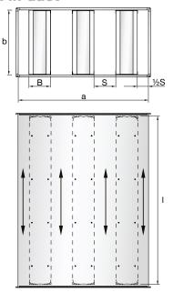
Length of splitter should be 50 mm shorter than length of duct.
